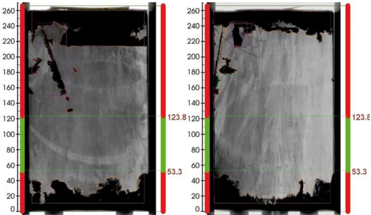
X-rays of silicon bricks in the infrared measuring station can detect contaminations, for instance inclusions of silicon carbide.
