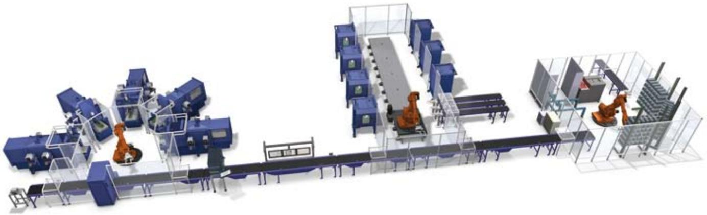
A fully automated production line for multicrystalline silicon bricks, with grinding, cutting (sawing) and gluing center.
